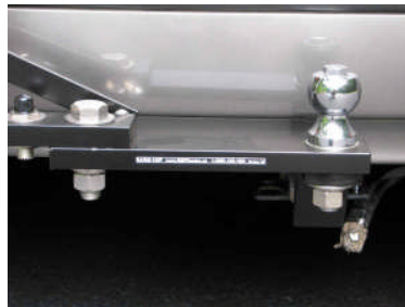
Figure 3: Same as Figure 2, except the HF antenna mount is turned 90 degrees and points backwards. If used with a trailer, be sure that the trailer does not contact the mount with this configuration!
