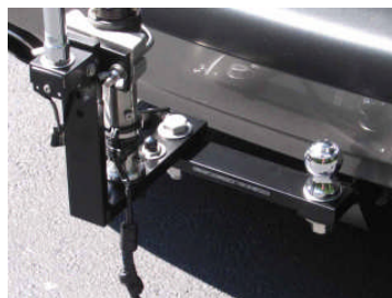
Figure 4: The Series 12 bare aluminum SARM with a bike rack on a vehicle with a Hi Q Antennas 5/160 antenna. The SARM is mounted to the hitch with the bolt that mounts the bike rack to the hitch.
