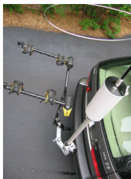
Figure 4: The Series 12 bare aluminum SARM with a bike rack on a vehicle with a Hi Q Antennas 5/160 antenna. The SARM is mounted to the hitch with the bolt that mounts the bike rack to the hitch.
