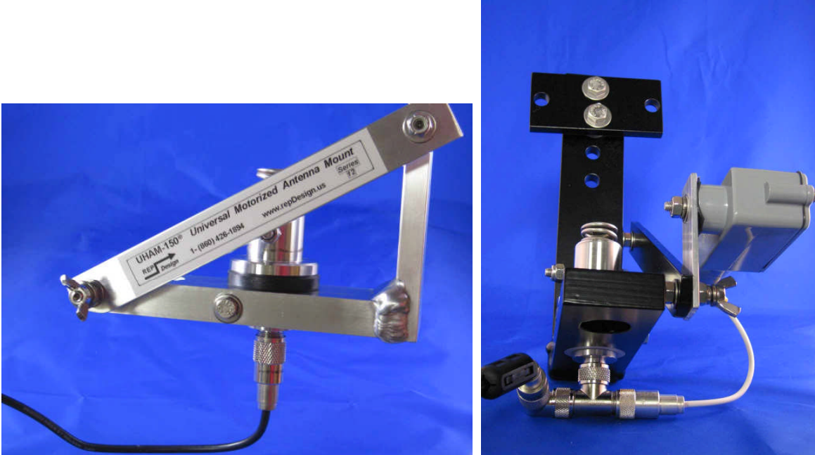
Figure 5: The photo below shows the SHD with a “matte black” powder coated UHAM-150 mount – the silver area around the base of the SHD is masked off during powder coating to ensure a “bare metal” mounting surface for the SHD. It is very important to ensure a good ground - if your mount is painted or has a non-conductive coating, this coating MUST be removed between the SHD and the bottom of your mount. This photo also shows an example of a second point of attachment that is required for medium and larger antennas if mounted to the SHD (or any SO239 antenna mount for that matter).
