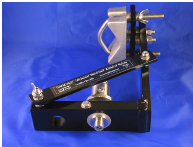
Figure 5: The photo below shows the SHD with a “matte black” powder coated UHAM-150 mount – the silver area around the base of the SHD is masked off during powder coating to ensure a “bare metal” mounting surface for the SHD. It is very important to ensure a good ground - if your mount is painted or has a non-conductive coating, this coating MUST be removed between the SHD and the bottom of your mount. This photo also shows an example of a second point of attachment that is required for medium and larger antennas if mounted to the SHD (or any SO239 antenna mount for that matter).
