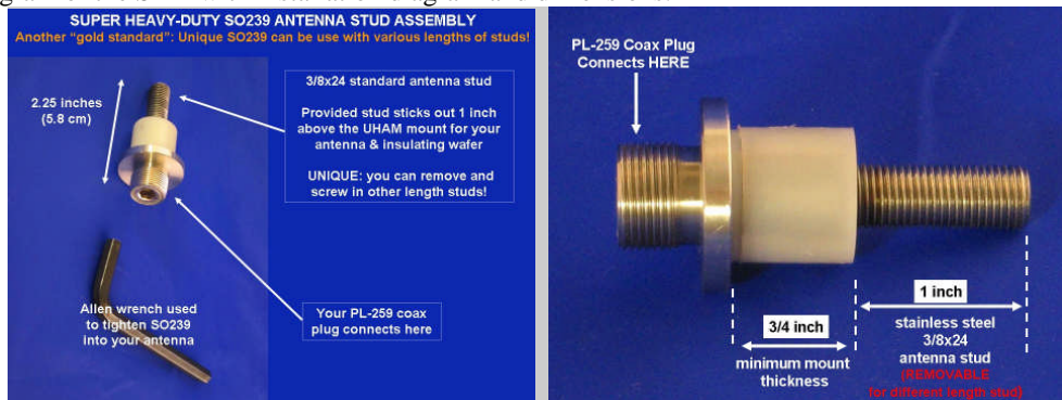
Figure 2: Diagram of the SHD with installation diagram and dimensions.
